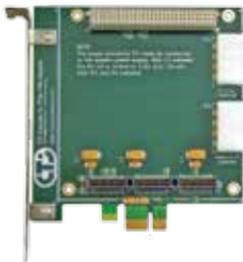
**PCI Express to PCIe/104 Adapter** allows a PCIe/104 or PCI/104-Express card to be installed into a standard PCI Express system slot.
