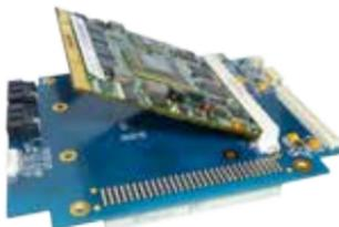
**Xtreme/SBC PCI-104 Single Board Computer** utilizes the PCI-104 form factor, supporting four peripheral boards. Instantly access a variety of features using the SBCs on-board connectors. Embedded processor options include AMD Fusion/G-Series, Intel® Atom™ Z500 & E600, Freescale i.MX51 & i.MX6, Texas Instruments OMAP, NVIDIA Tegra and VIA Nano E-Series.
