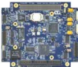
**Xtreme/SBC PCIe/104 Single Board Computer** utilizes the PCIe/104 form factor with 4 x1 PCIe lanes. Instantly access a variety of features using the SBCs on-board connectors. Embedded processor options include AMD Fusion/G-Series, Intel® Atom™ Z500 & E600, Freescale i.MX51 & i.MX6, Texas Instruments OMAP, NVIDIA Tegra and VIA Nano E-Series.
