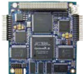
**ComSync/PCI-104** which is based on the PCI bus, is a two-channel, multi-protocol serial adapter which offers high performance, reliable, synchronous or asynchronous serial communications.
