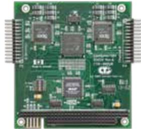
**ComSync/104** offers two synchronous/asynchronous RS-232, RS-422, RS-449, EIA-530, EIA-530/A, V.35 and X.21 serial channels.
