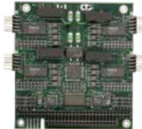
**Xtreme/104 Opto** offers two or four asynchronous serial ports with 3kV optical isolation on all signals and ports.
