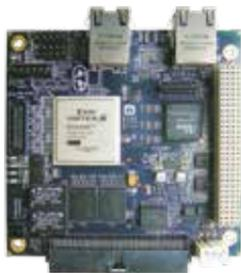
**FreeForm/PCI-104** is a reconfigurable FPGA development board with high speed digital I/O that combines a user programmable FPGA with a 32-Bit, 33MHz PCI-104 interface.
