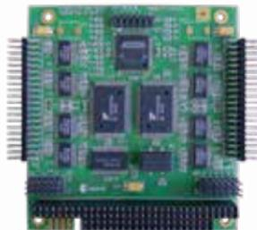
**Xtreme/104 RS-232** offers four or eight asynchronous RS-232 serial ports.
