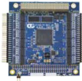
**Xtreme I/O Opto** is a 48-bit isolated digital input/output board with 24 optically isolated inputs and 24 optically isolated outputs.
