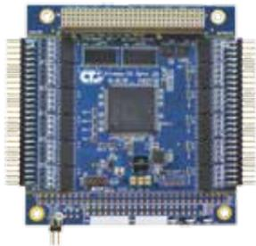
**Xtreme I/O Opto** is a 48-bit isolated digital input/output board with 24 optically isolated inputs and 24 optically isolated outputs.
