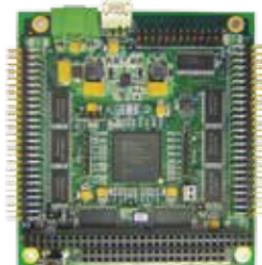
**FreeForm/104** is a PC/104 based FPGA development board for digital I/O and control applications.
