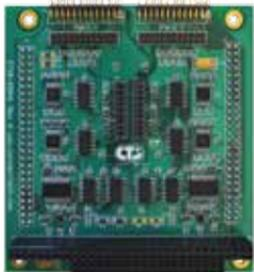
**FreeForm/104 Daughter Board** is a FreeForm/104 adapter board that enables users to capture and process synchronous and asynchronous RS-232 or RS-422/485 serial data with customizable FPGA implementations.
