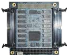
**Xtreme/104-Plus 16 Port** offers 16 ports of switchable RS-232/422/485 on a single PC/104-Plus card. This provides the highest port density and most flexible PC/104-Plus serial port solution available.
