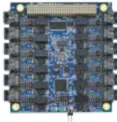
**Xtreme/PCI-104 Opto 12 Port** offers 12 ports on a PCI-104 card, with the added protection of 1kV optical isolation on a rugged and compact form factor.
