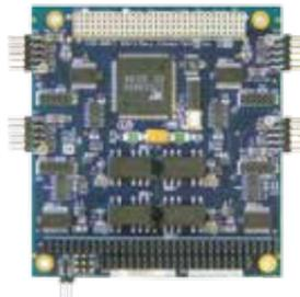
**Xtreme/104-Plus Opto** provides the added protection of 3kV optical isolation on a rugged and compact form factor for critical embedded applications.
