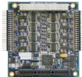
**Xtreme/104-Express** is a PCI/104-Express multi-port serial board which provides a PCI-104 pass-through connector. Fully PCI/104-Express compliant.
