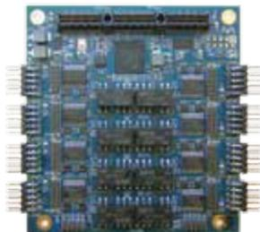
**Xtreme/104-Express Opto** is a PCIe/104 serial card with 3 kV optical isolation for rapid data transfer and high reliability.
