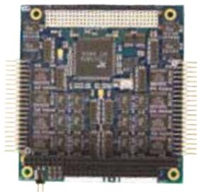
**Xtreme/104-Plus** offers 4 or 8 high speed asynchronous RS-232/422/485 ports, 8 selectable RS-232/422/485/UTL ports, or 2/4 dedicated RS-423 ports.
