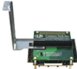
**PCIe/104 to PCI Express Adapter - Top Stacking** model allows a PCI Express card to be installed into a PCIe/104 or PCI/104-Express single board computer system in a stack up configuration.
