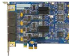
**BlueStorm/Express Opto** is a standard profile PCI Express serial card which offers 4 ports of RS-232/422/485 connectivity, and 3kV optical isolation. These x1 lane cards are compatible with x1, x4, x8, x16 lane PCI Express slots.
