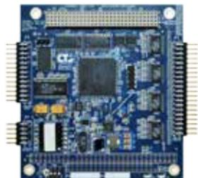
**Xtreme I/O ADC-DAC** is an analog data acquisition board for the small form factor embedded market place.
