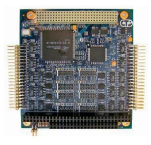
Connect Tech's Titan/104-**Plus** combines the best in performanace and design of full sized PCI bus devices with the rugged and compact form factor of PC/104.
