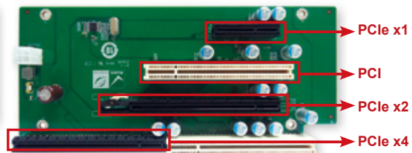
• One PCIe x 1 (physical one PCIe x4 slot) and one PCIe x2 (physical PCIe x16 slot) and one PCI
