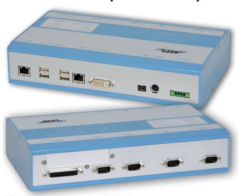
PIP19 dimensions: 270 x 162 x 62 m (L x W x H). Weight 2.2kg, rugged aluminum housings with best EMI/RFI protection (inside chromated, externally powder coated or eloxated)
